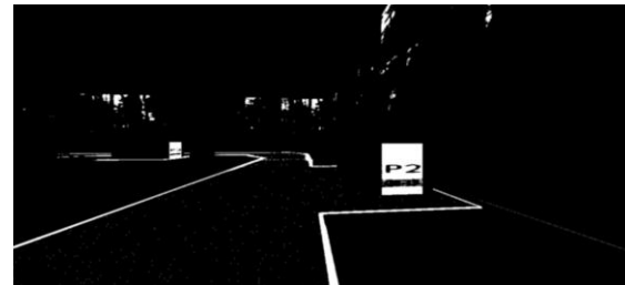
HSV filtered camera view for self-driving
